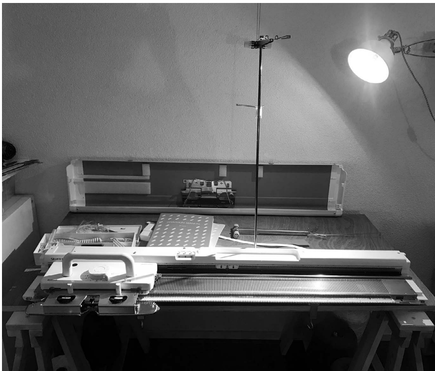
Figure 12.4 SilverReed SK840 domestic knitting machine.
