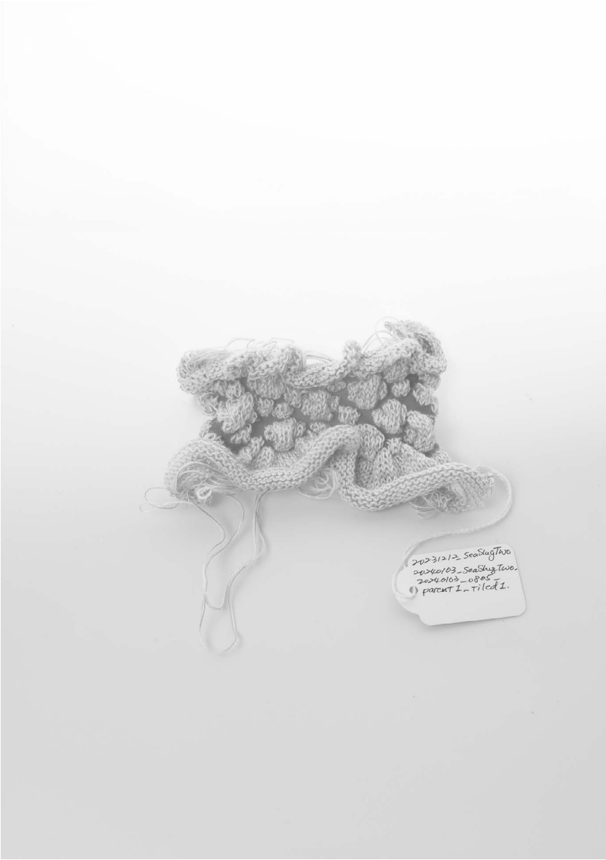
Figure 12.10 The knit side of the pattern shown in Figure 12.9 , knitted with yellow elastic yarns with cotton-acrylic yarns.
